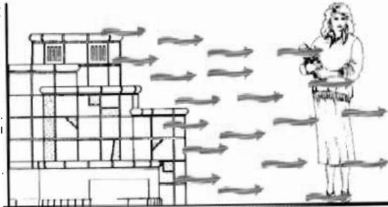
Radiant heating systems reduce these problems, as the air no longer becomes the sole means by which heat is transferred.
