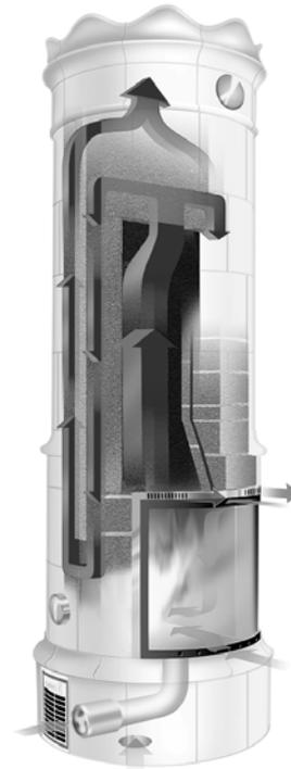
The smoke canals are made of high-density composite stone such as olivine, which has excellent heat absorption qualities and high heat storage capacity.
