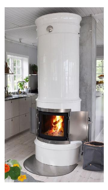
Technical data Article no. G350 CE marking: EN 15250 Height: 2290 mm (customised to your needs) Weight: 1,300 kg Diameter (base): 770 mm Energy efficiency: 92.4% Nominal heat output (kW): 4.5 Heat retention: Up to 24 hours Connection: Rear or top flue connection
